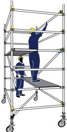
, Install a temporary platform between the two Base Frames at approximately 1.0m high. Then install the Trapdoor Platform between the two frames at at approximately 2.0m high, offset from the first platform.
