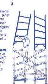
6. Fit the PLAIN **PLATFORM** first, then the WALK-THROUGH **PLATFORM** with the hinges of trapdoor to the outside of tower. Insert the **GUARD RAIL FRAMES** into the top of the last frame.
