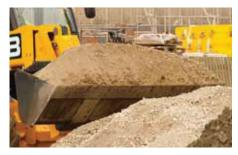
GENERAL PURPOSE SHOVEL JCB-designed for maximum performance and durability Drilled to accept toeplate or teeth Quickhitch compatible Loadalls' excellent shovel capability
