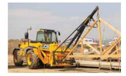
TRUSSMASTER The safe alternative to manual handling In placement mode the manual option has four fixed setting points, hydraulic option offers "inching" control The travel mode incorporates a steadying yoke for greater site safety
