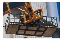
MAN PLATFORM Available factory fitted for 540-140 and 540-170 Full radio remote control of boom functions as standard Maximum personnel working heights of 15.11m to 18.12m with 300kg payload Platform widths up to 4 metres Optional 180° slewing for maximum flexibility
