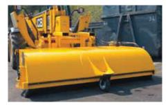
SWEEPER COLLECTOR Heavy-duty one piece canopy for maximum durability Class-leading visibility Floating mounting frame for increased sweeper output Combination steel and polypropylene brush Quickhitch or fork mounted fitment
