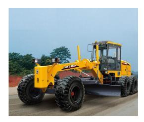
CUMMINS diesel engine (Tier3), low noise, low emmission. Electronic-hydraulic control power shift gearbox is used. The rear axle is three stage equipped with no-spin differential locking device creating steady and reliable driving. Fitted with a ROPS & FOPS cabin with electric wipers, mist eliminator and cold and warm air-conditioner.
