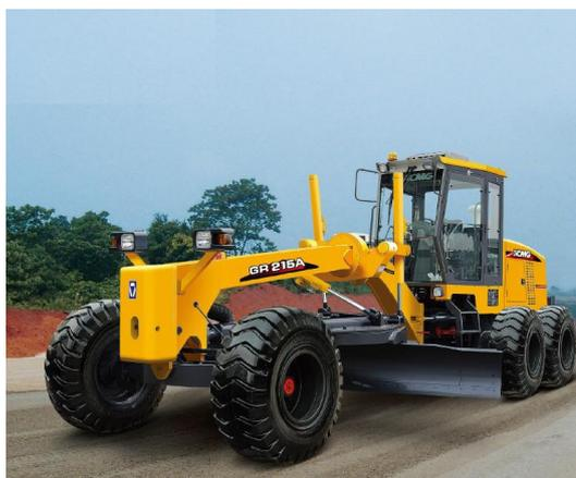
CUMMINS diesel engine (Tier3), low noise, low emission. Electronic-hydraulic control power shift gearbox is used. The rear axle is three stage equipped with no-spin differential locking device creating steady and reliable driving. Fitted with a ROPS & FOPS cabin with electric wipers, mist eliminator and cold and warm air-conditioner.
