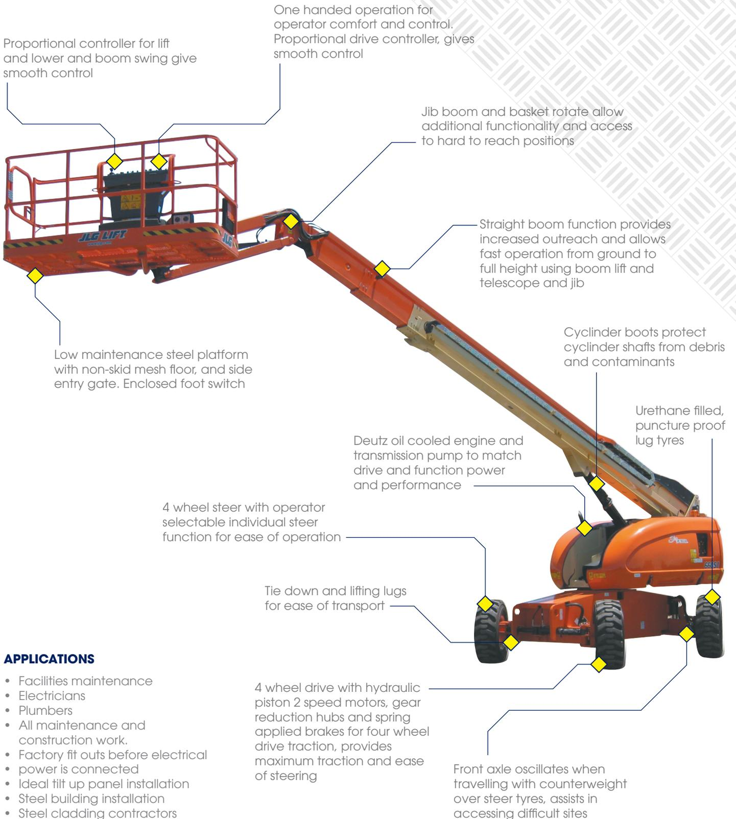
Proportional controller for lift and lower and boom swing give smooth control
